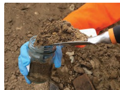
Spoil and water from below the slab should be assumed SCW unless tested otherwise
