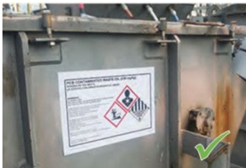
PCB waste labelled ready for collection
