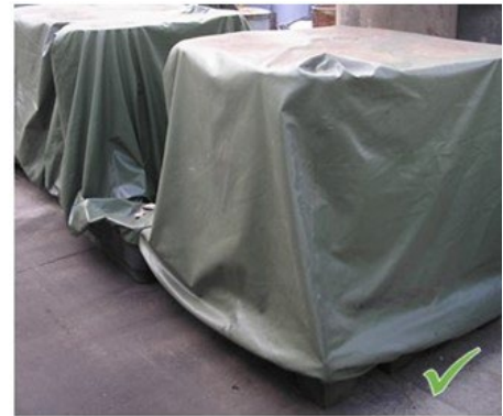
Bunded pallets should be covered when exposed to the weather
