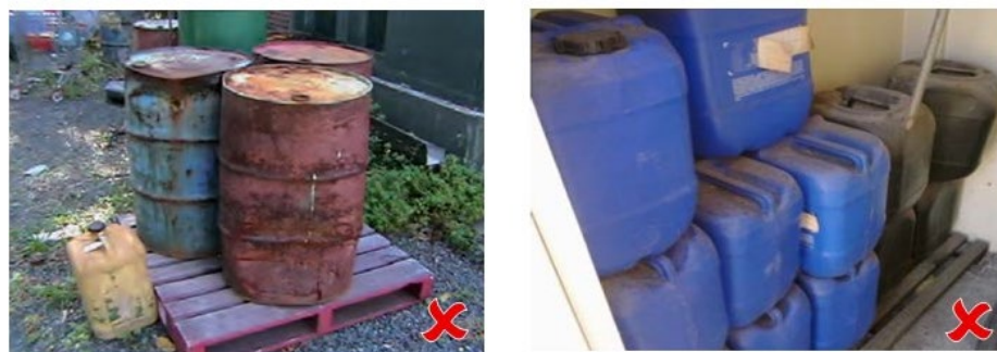
Drums in poor condition, not banded, unlabelled or uncovered can leak and contaminate land or waterways
