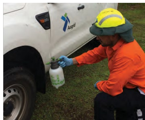
Plant and equipment need to be disinfected before entering native bushland or leaving infested areas
